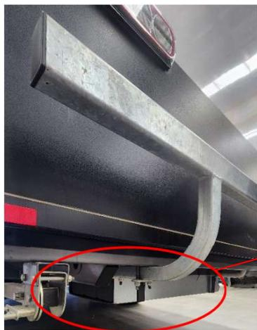
Bumper bar secured with U-Bolts to the chassis
