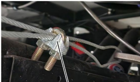
Reinstall the handbrake cable
